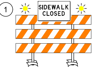
TYPE III BARRICADE CLOSURE W/ ORANGE SAFETY FENCE AND R9-9
